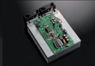
PA Unit with a Large Heatsink
